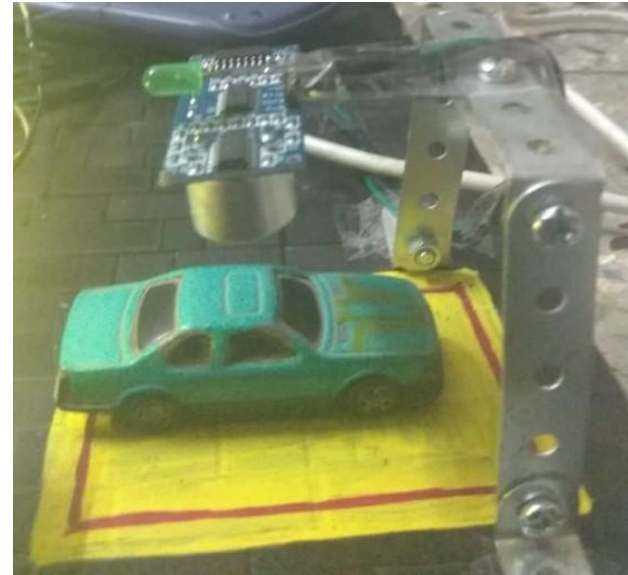
Figure 12. LED light off slot 1 (busy)
