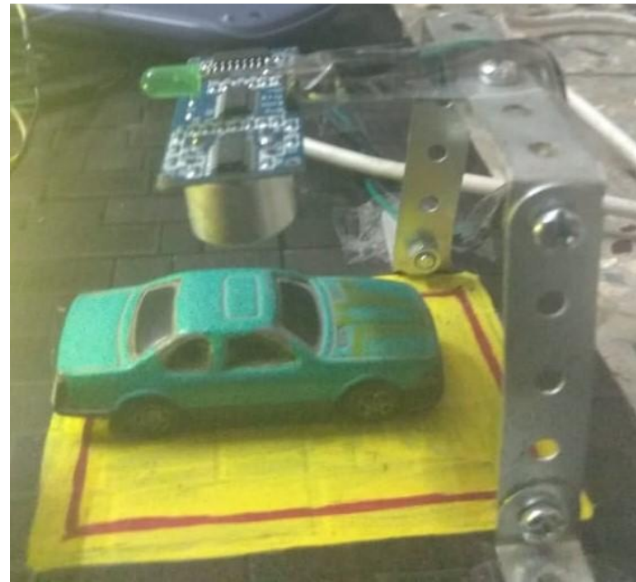
Figure 20. LED light off slot 1 (busy)
